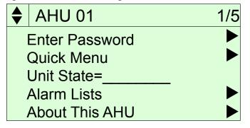
The password field initially has a value \*\*\*\* where each \* represents an adjustable field. These values can be changed by entering the Edit Mode described below.
