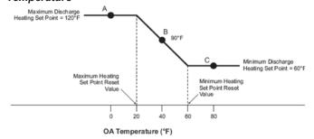
Whenever the Htg Reset Type or Engineering Units is changed, the Min Htg Spt @ and Max Htg Spt @ values revert to default values as follows:
