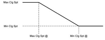
When Airflow is selected, the values "Min Clg Spt @" and "Max Clg Spt @" are entered as percentage values. When Ext mA is selected, the values "Min Clg Spt @" and "Max Clg Spt @" are entered as mA values. When Ext VDC is selected, the values "Min Clg Spt @" and "Max Clg Spt @" are entered as VDC values.
