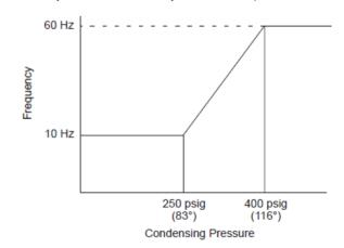
Figure 21: Speedtrol Operating Characteristics (for Variable Speed Inverter Compressor Units with Start-Stop Control)
