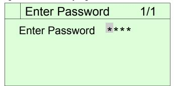
Entering an invalid password has the same effect as continuing without entering a password. Once a valid password has been entered, the controller allows further changes and access without requiring the user to enter a password until either the password timer expires or a different password is entered. The default value for this password timer is 10 minutes. It is changeable from 3 to 30 minutes via the Timer Settings menu.
